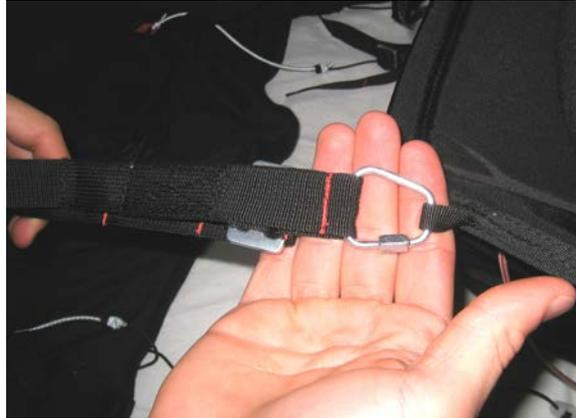
Then hook the loops on the upper straps to the main karabiners, ensuring that the pulleys and the adjustment straps are facing inside. We recommend turning the karabiners so that the locking collar faces the pilot, as shown in the photo.
