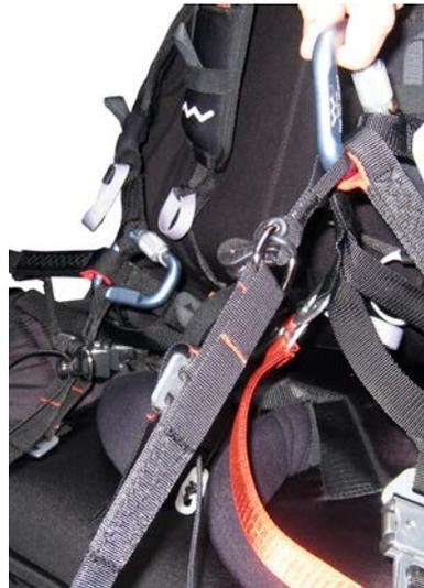
Pass the Lycra over the karabiner, so that it covers all the straps. When performing this operation, it may be necessary to remove the karabiner from the harness. In this case, make sure that you reassemble all the straps to the karabiner in the correct order.
